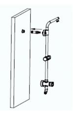
2. Align the top mount of slide bar with the connector and press it firmly until the escutcheon (flange cover) is flush with the wall.
